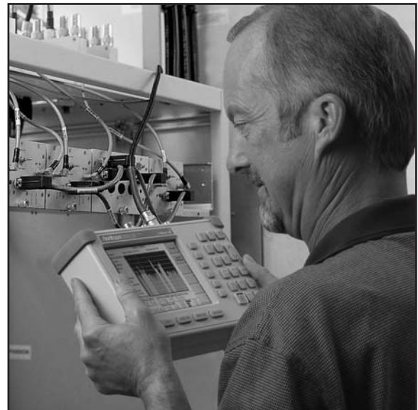
Figure 6. Cell Master can demodulate the CDMA signal by connecting to the base station.
