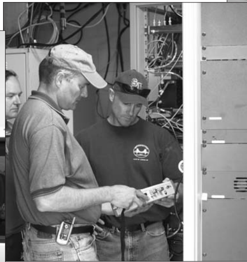
Figure 4b. The Cell Master MT8212B can measure CDMA performance via Direct Connection to the base station.
