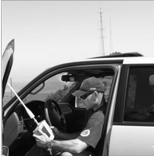
Figure 4c. The Cell Master MT8212B can measure CDMA performance Over The Air (OTA) with an antenna.
