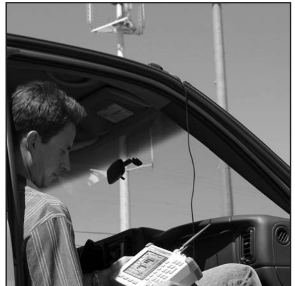
Figure 8. The Cell Master MT8212B can also demodulate the CDMA signal using an over the air antenna. A built-in GPS feature provides users with UTC time and location information.
